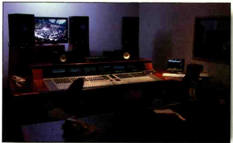
The Euphonix C-5 systems in the two Production Audio Control Rooms provide a base from which all originating sources can be 24-bit and support up to a 96kHz sampling rate for live and post production.
